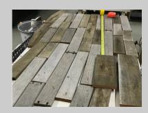
I ran the wood through my planer to remove the weathered surfaces and. cut off the ends where the screw holes had been. Then scratched my head trying to decide what to do with this newly salvaged teak.
