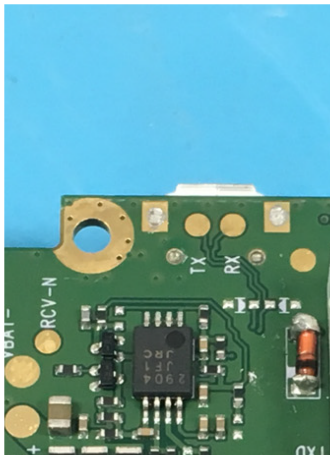
Reverse of the micro USB port has test pads labeled RX and TX
