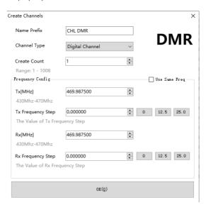
The prefix name of the channel can be set on the bar of the Name Prefix. When the channel is created, it will automatically add a digital index number for it. There are two options for the Channel Type, that is, Digital Channel and Analog Channel. The Create Count determines how many channels are created.
